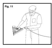
22. Do not overreach. Keep proper footing and balance at all times when using or handling the tool.
